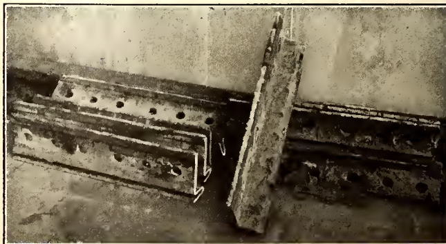
WORN ANGLE BARS BEFORE BEING RECLAIMED BY ELECTRIC WELDING
